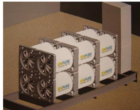
A basic system, consisting of modules arrayed on a skid (Figure 4), can form the basis for system integrators to construct systems for specific applications by adding the required piping, instrumentation, controls and power supply. Direct shipment of the basic system from the factory to site is possible, with final assembly on site [1].
