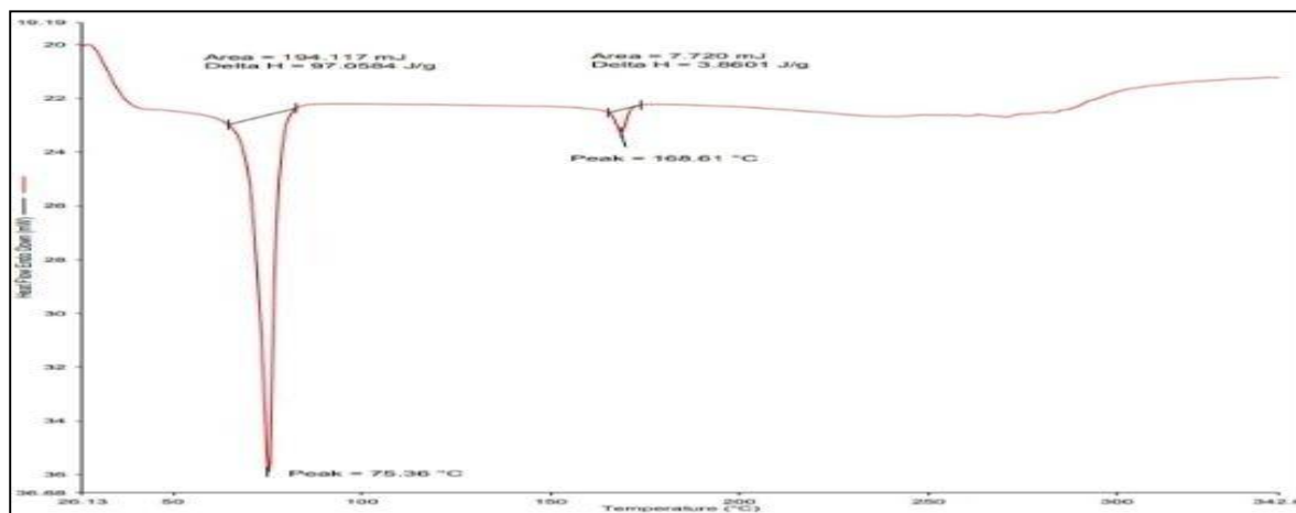
Figure 4: DSC of Compritol 888ATO+Atomoxetine hydrochloride
