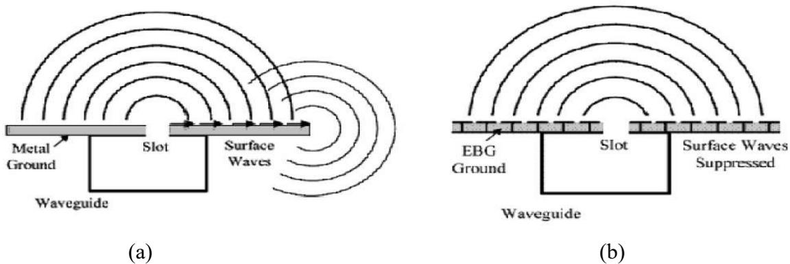
Figure 5: substrate without EBG structure (a) and with EBG(B).
