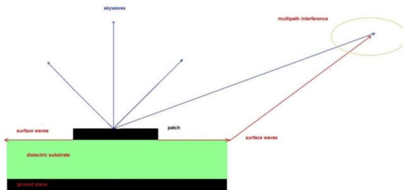
Figur4:Sky waves, surface waves and multipath interference in patch antenna.
