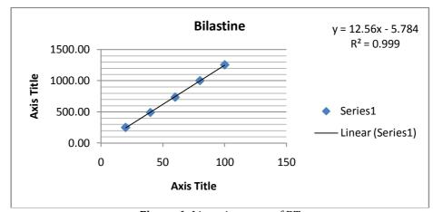
Figure 6: Linearity curve of BT
