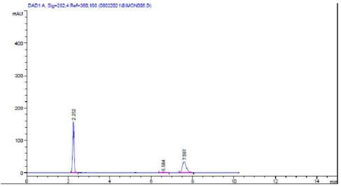
Figure. 10:Chromatogram of mixture of BT and ML degraded with neutral hydrolysis
