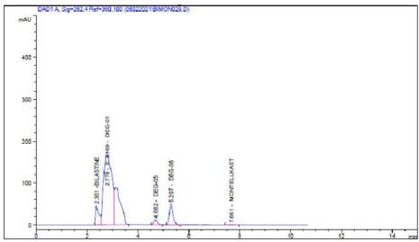
Figure. 11:Chromatogram of BT and ML degraded with oxidative hydrolysis
