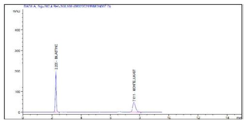
Figure 5: Chromatograph of mixture of sample BT and ML
