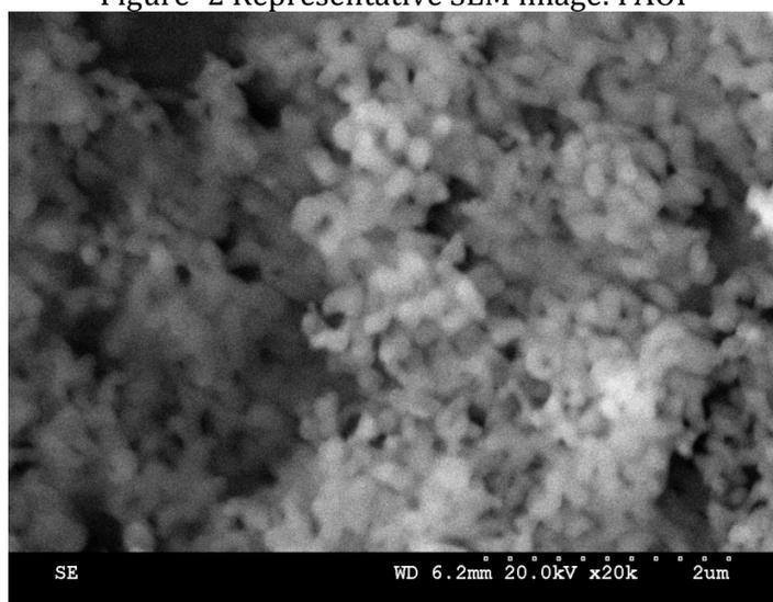
The above photograph is the SEM of Al<sub>2</sub>O<sub>3</sub> of 150 nm nanoparticle
