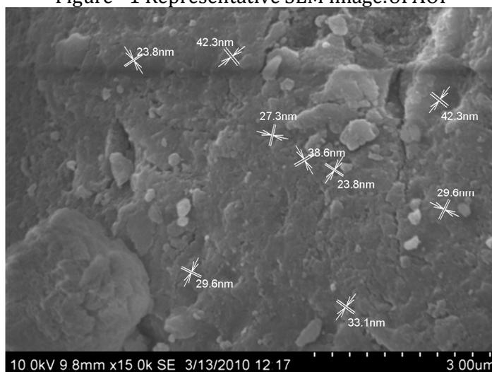
The above photograph is the SEM of Al<sub>2</sub>O<sub>3</sub> of 10 nm nanoparticle.
