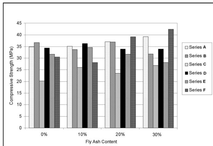
Fig. 2. Compressive strength with varying fly ash contents.
