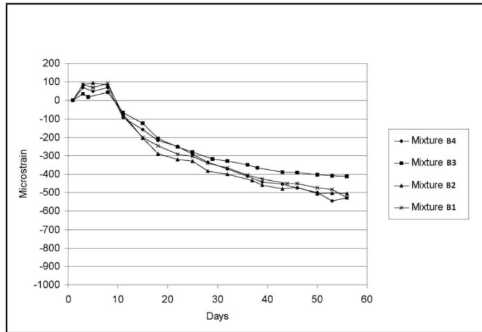
Fig. 4. Shrinkage strains for mixtures from Series B.
