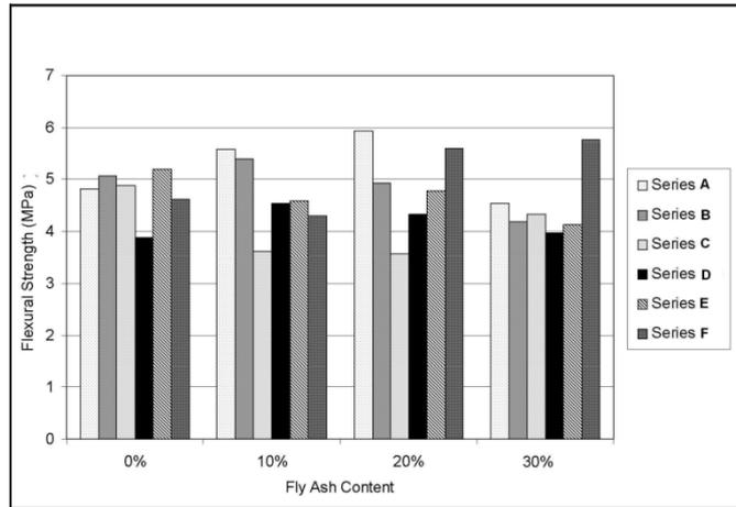
Fig. 1. Flexural strength with varying fly ash contents.
