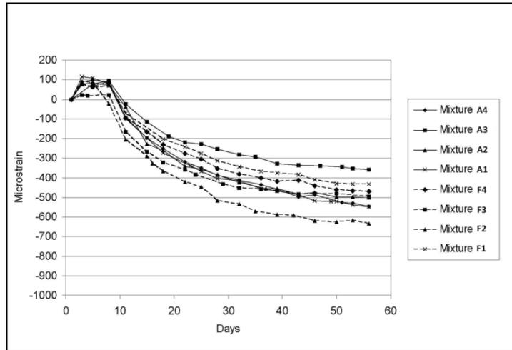
Fig. 8. Shrinkage strains for mixtures from Series F compared to mixtures without fibers.
