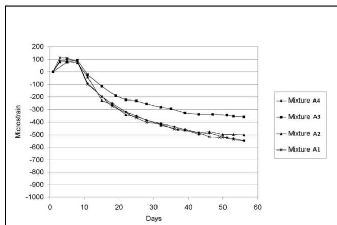
Fig. 3. Shrinkage strains for mixtures from Series A.
