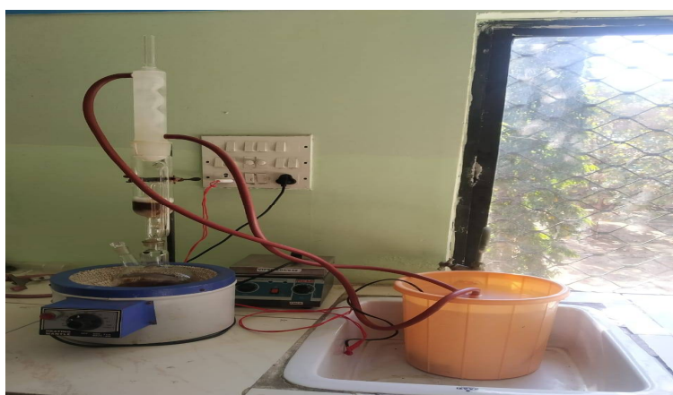
Fig no: 6 Cyperus Rotundus Extraction by Using Ethanol as Solvent
