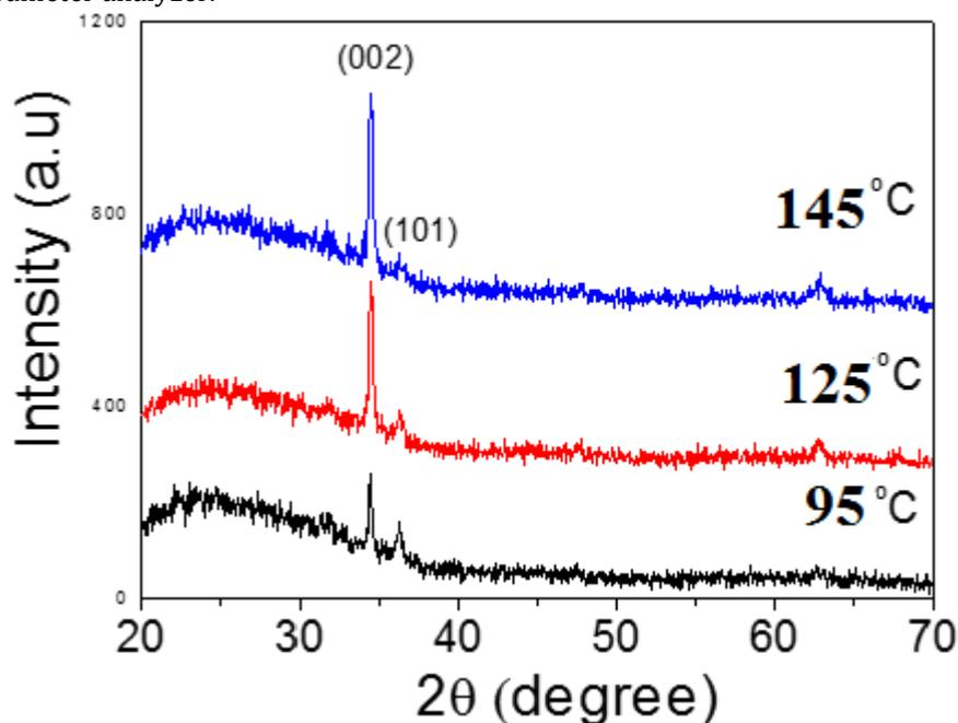
Fig. 1 XRD patterns of ZnO thin films under various temperature treatments.
