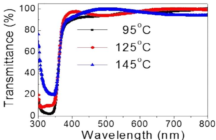
Fig. 3 The optical transmittance spectra at different rinsing temperatures.
