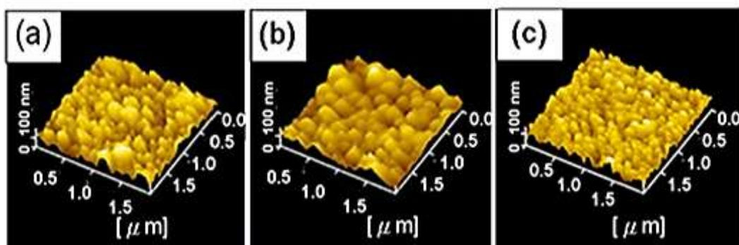
Fig. 2 AFM image of the ZnO channel layer at temperatures of (a) 95 °C (b) 125 °C, and (c) 145°C.
