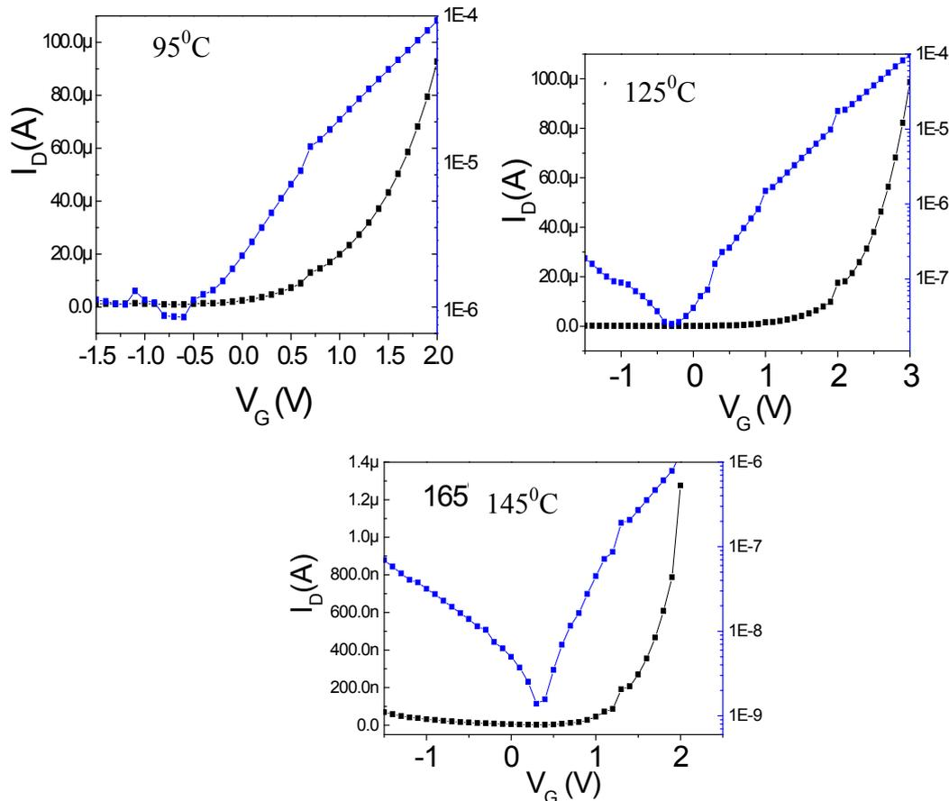
Fig. 5 Transfer characteristics of SILAR ZnO TFT at various temperatures.
