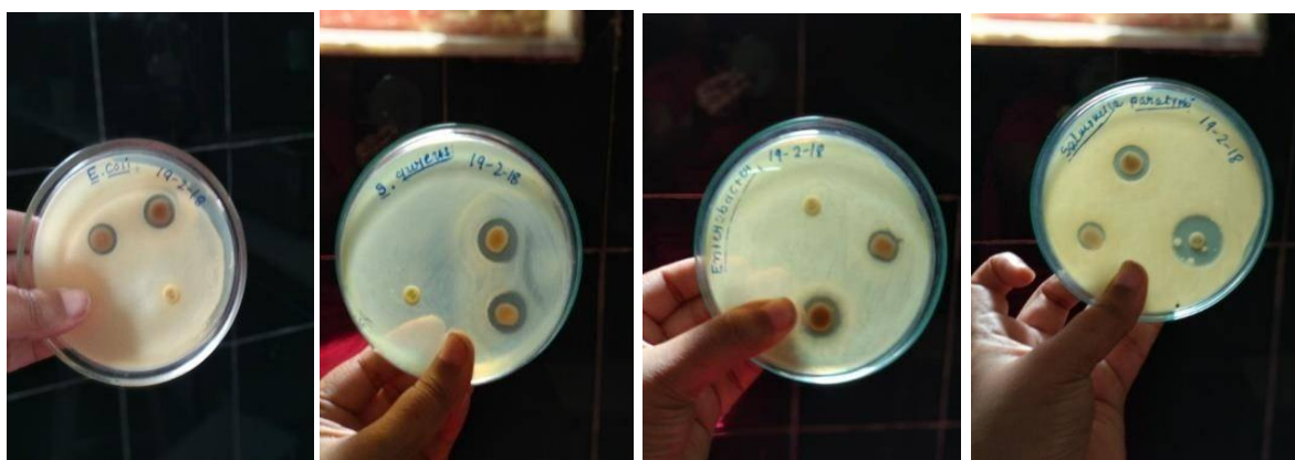
Picture 1.: Pictorial depiction of antimicrobial activity of film against four food borne Pathogens: 1) E. coli 2) S.aureus 3) E.aerogenes 4) S.typhi
