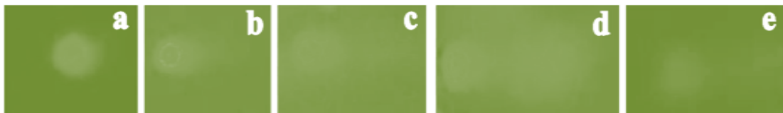
Figure.3. Images of Classes of Comet events: a) Class 1 - no damage, <5%; b) Class 2 - low level damage, 5–20%; c) Class 3 - medium level damage, 20–40%; d) Class 4 - high level damage, 40–95%; e) Class 5 - total damage, >95%.
