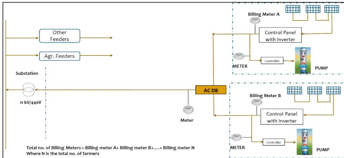
Figure 1: System Configuration of Proposed Solar PV based Mini Grid
