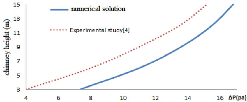
Figure 12 the effect of height on the suction chimney insulation
