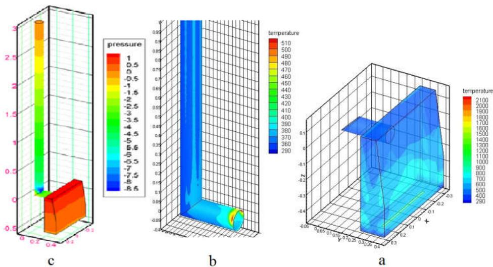
Figure (6) a) furnace heater temperature contour, b) the first one -meter of chimney temperature contour, c) contour of the furnace and chimney pressure at sea level with a smooth internal surface
