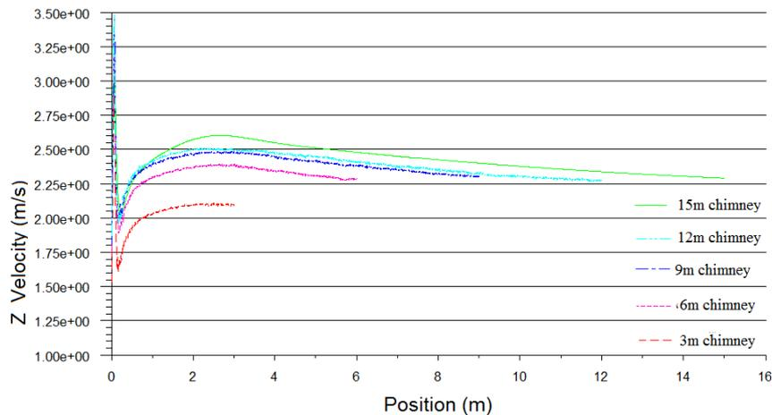
Figure (19) Central line speed type 1 chimney with different heights
