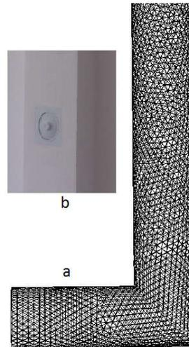
Figure 2 (a) studied chimney mesh and chimney inlet view, (b) actual operation of chimney inlet
