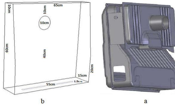
Figure 1 (a) Real heater furnace, (b) Studied simplified model
