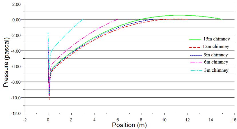
Figure (18) Central line pressure type 1 chimney with different heights
