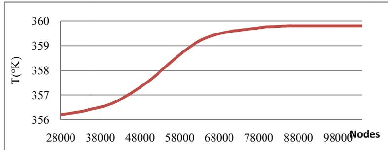
Figure 4 Effect of different mesh on 3-meter chimney exhaust gas temperature
