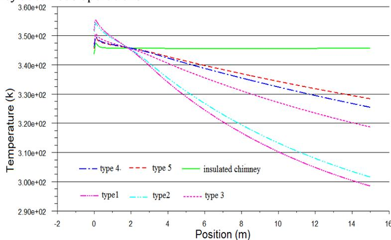
Figure (17) the temperature in central line 15 meter chimney in different operations
