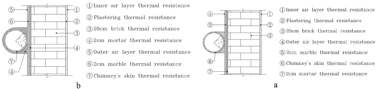
Figure 9 A) operation details chimney type 1, B) operation details chimney type 2
