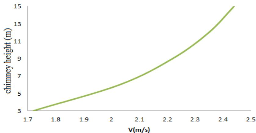
Figure (13) the effect of height on the average speed of the exhaust chimney insulation
