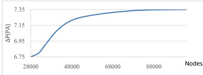
Figure 3 Effect of different mesh on 3-meter chimney suction
