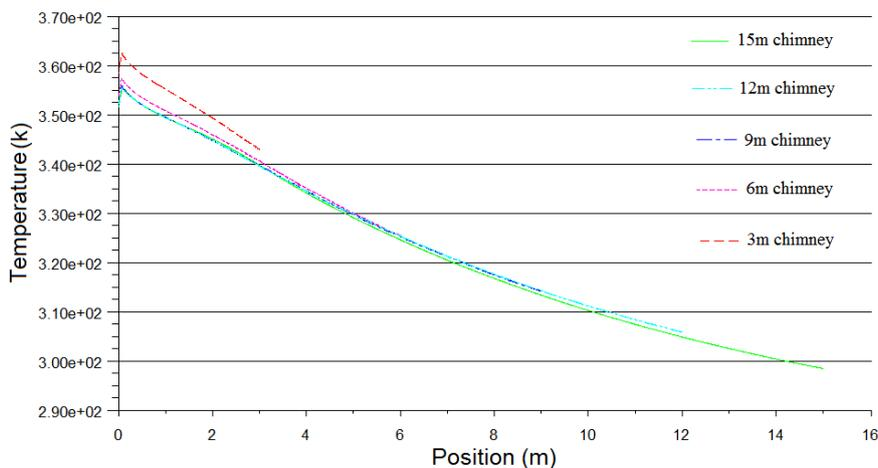
Figure (20) the temperature of the flue type 1 chimney with different heights
