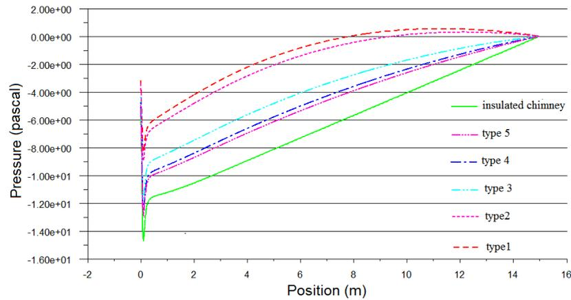
Figure (15) Central line pressure in 15 meters chimney in different operations
