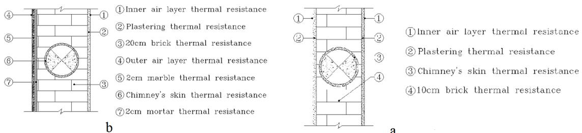
Figure 11 (A) operation details chimney type 4, B) operation details chimney type 5
