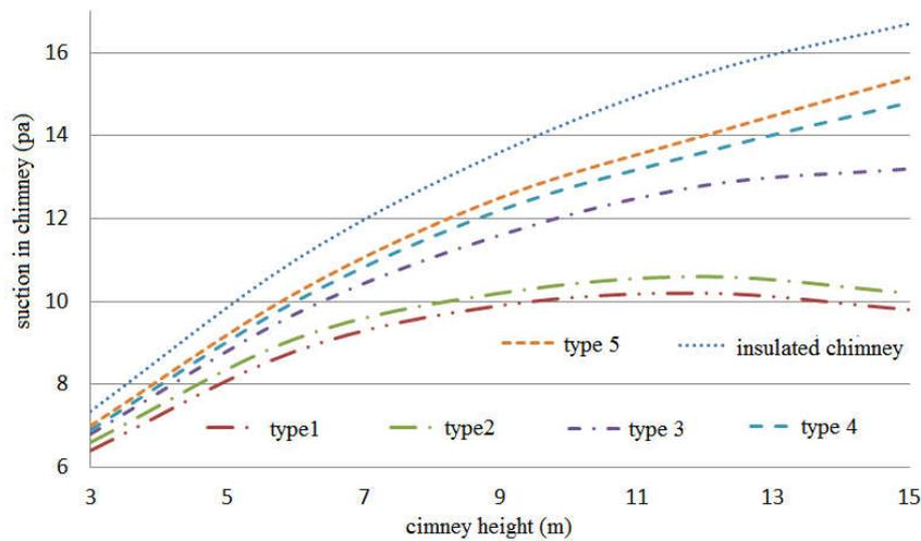
Figure (21) suction in the chimney with different lengths and different operation
