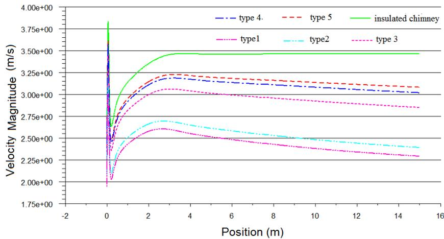
Figure (16) Central line speed in the 15-meter chimney in different operations
