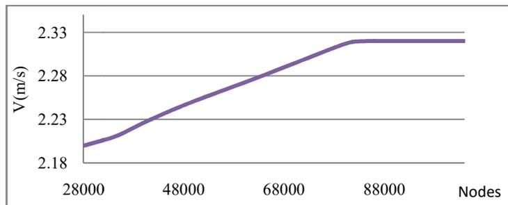
Figure 5 Effect of different mesh on 3-meter chimney emissions speed
