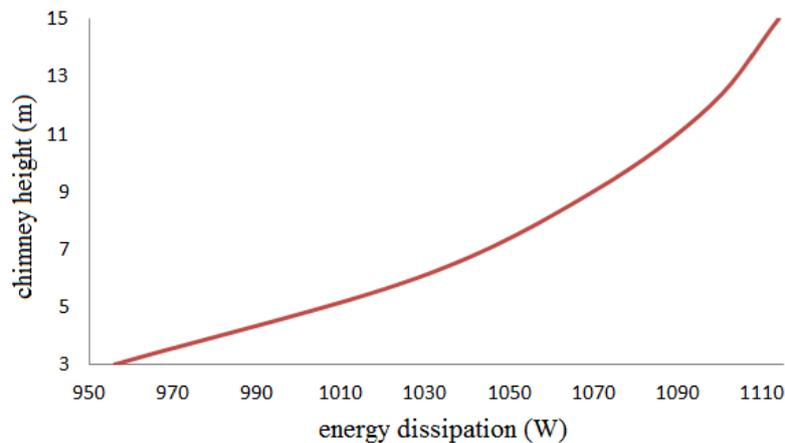
Figure (14) the effect height on the rate of energy dissipation along the chimney exhaust
